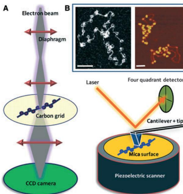
**Fig. 1.** Molecular microscopy: the two main devices. (A) Transmission electron microscopy (TEM) and (B) atomic force microscopy (AFM) both enable the visualization of nucleoprotein complexes at a nanometric scale. Insert: TEM (left) and AFM (right) images of nucleosomal arrays reconstituted with purified histones on bacterial plasmids (scale bars = 50 nm).
